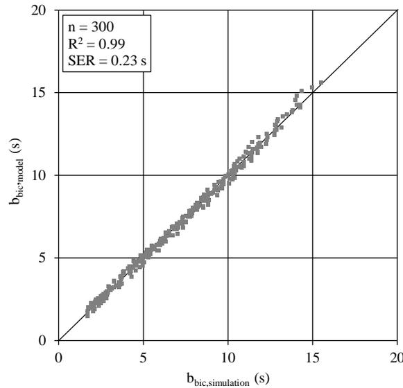
**FIGURE 12: Comparison of the simulated and the calculated blockage times with equation (8) and  $b_{P,bic} = 0.557$  s,  $b_g = 3.497$  s and  $k = 0.887$  for  $v_{C,bic} = 1$  to 7 bicycles**
