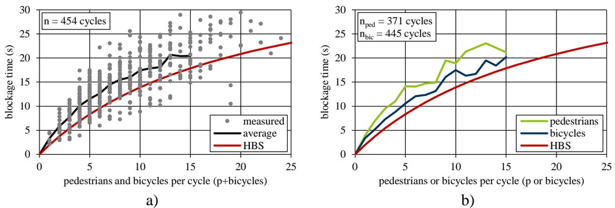
**FIGURE 3: Empirically measured blockage times  $b$  at the example crossing as a) the total blockage time and b) the separately measured blockage time of pedestrians and bicycles**
