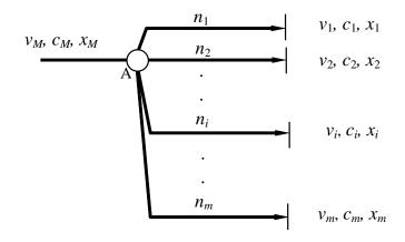
FIGURE 3 - Relationship between a shared lane and its sub - movements
