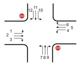
FIGURE 1 - Definition of movements at an unsignalized intersection in the HCM 2000
