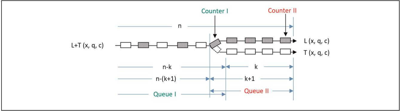
Figure 6. “Two-queue” system at a shared short lane: Queue I: M/G/1, Queue II: M/M/1 (cf. Wu and Brilon, 2019 [14]).
