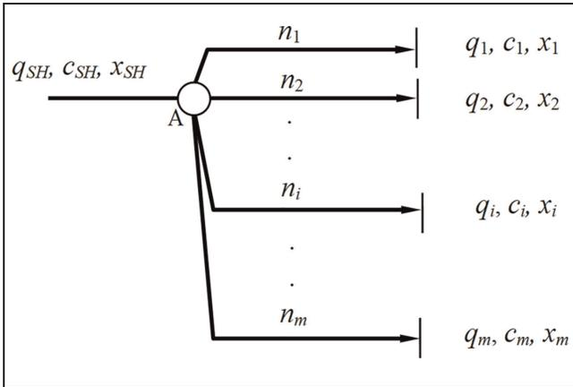
**Figure 4.** Relationship between a shared lane and its sub-movements (cf. Wu, 1999 [12]).
