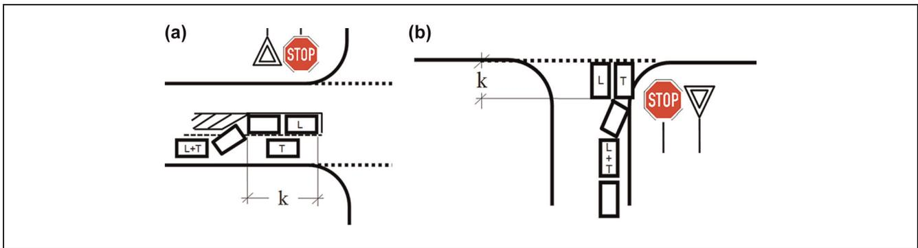
**Figure 3.** Possible queues and lane configurations at approaches of two-way-stop-controlled intersections: (a) major approach, (b) minor approach (cf. Wu, 1999 [12], Wu and Brilon, 2010 [13]).
