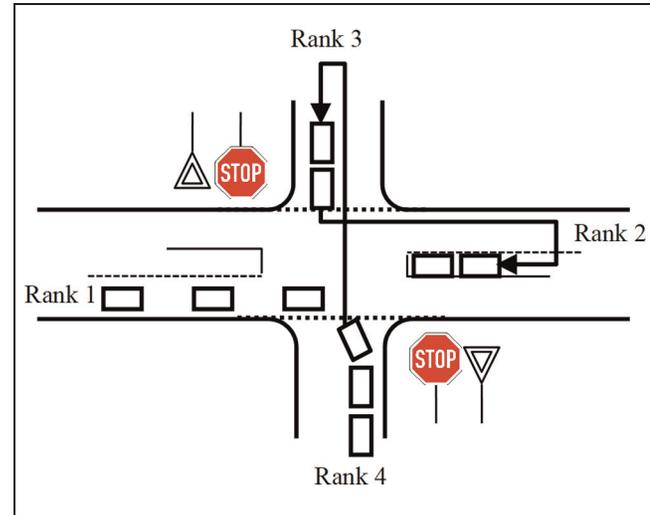
**Figure 1.** Queues in movements of different ranks and the operation sequence (cf. Wu, 1998 [11]).
