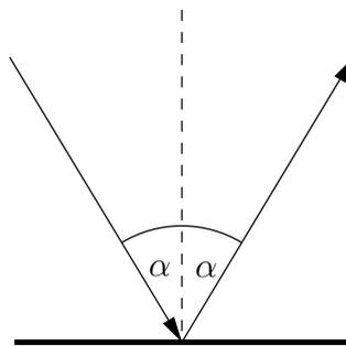
Figure 2: Reflection: The angle  $\alpha$  of the incoming ray is equal to the angle of the reflected ray.
