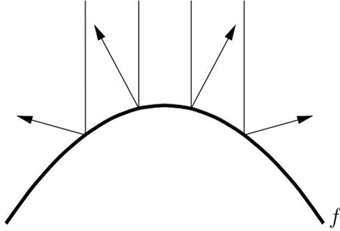
Figure 4: A solution  $f$  which does not fulfill the initial requirement. While  $f$  does have a unique focal point, it is “on the wrong side”.
