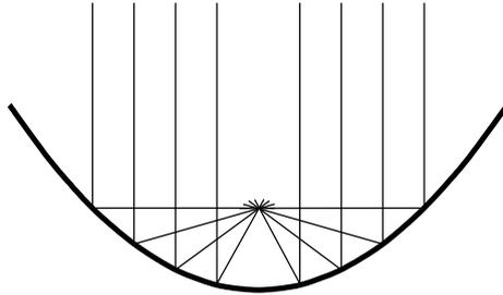
Figure 1: A parabolic mirror bundling incoming parallel rays into a focal point
