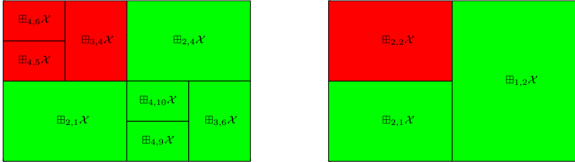
Figure 2: Hyperrectangular state space partitions that correspond to the binary tree in Fig. 1. Every hyperrectangle \boxplus_{\delta\beta}\mathcal{X} uniquely corresponds to its node (\delta, \beta) . The partition on the left belongs to the leaf node representation (underlined nodes in Fig. 1). The more compact partition on the right corresponds to the nodes labeled with an asterisk in Fig. 1.
